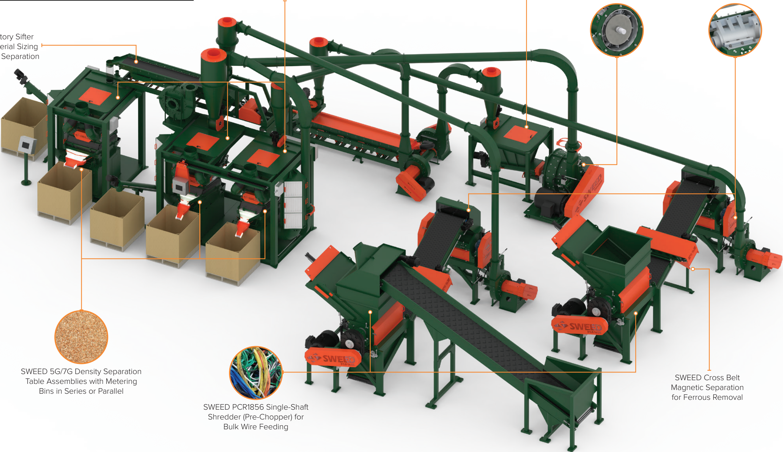
SWEED Separation Table Mounted, Auger Driven Metering Bin
