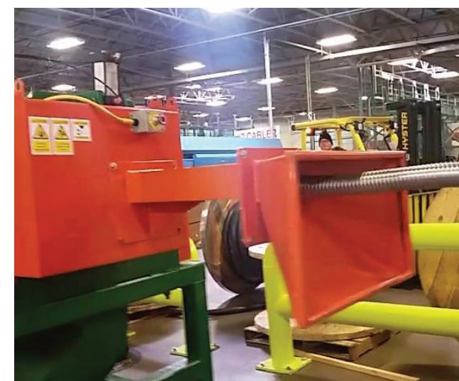
Large BX Cable being despoiled and chopped by SWEED’s 5703 XHD
