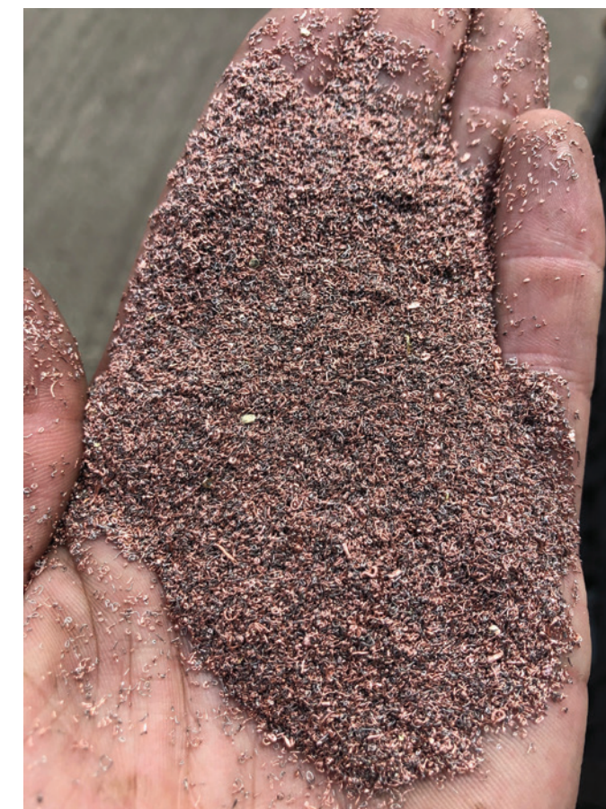
The end product from mixed low yield ICW after running through SWEED Turbo Mill.
