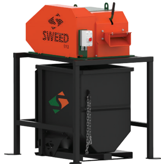
The Model 513 is shown sitting on and over an optional basic stand and 1/2 yard self-dumping hopper.
